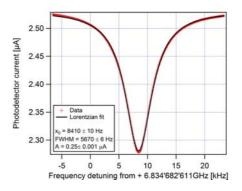
Fig. 5. DR clock signal obtained with the  $\mu\text{-LGR},$  with 5.67 kHz linewidth at 9.9% contrast.
