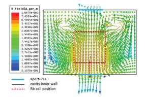
Fig. 2. Simulated magnetic field of the TE mode at 6.835GHz (t=2.0mm). The position of the micro-fabricated Rb vapor cell is indicated by the red dotted line.
