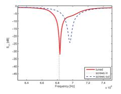
Fig. 4. Tuning of the µ-LGR prototype (t=2.0 mm) at 6.835 GHz.
