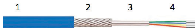
Fig. 3. The BRUsteel cable. From left to right: the nylon jacket (1), the inter-laced steel wires (2), the stainless steel loose tube (3), the four multimode fibers (4). In (3) is applied the electrical heating. From Brugg Cables ( http://www.bruggcables.com ), technical sheet of the BRUsteel fiber cable.
