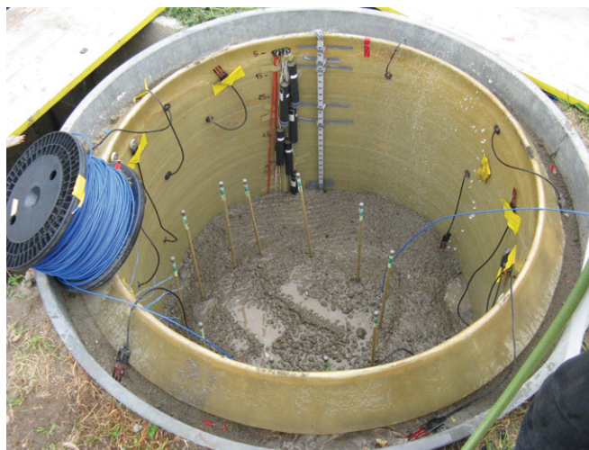
Fig. 4. Installation of the fiber optic cable. During uniform packing of the lysimeter, the soil is saturated and the fiber optic cable is wrapped around a bamboo-stick structure, which is removed after filling.
