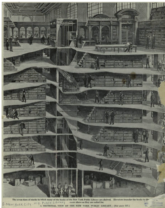
View of the stacks inside the Stephen A. Schwarzman Building from the May 27, 1911 issue of Scientific American . NYPL, Picture Collection
