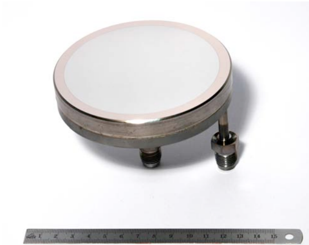
Fig.5.3.1 Prototype of ITER first mirror: rhodium or molybdenum thick reflective coating layers on stainless steel or TZM cooled blank
