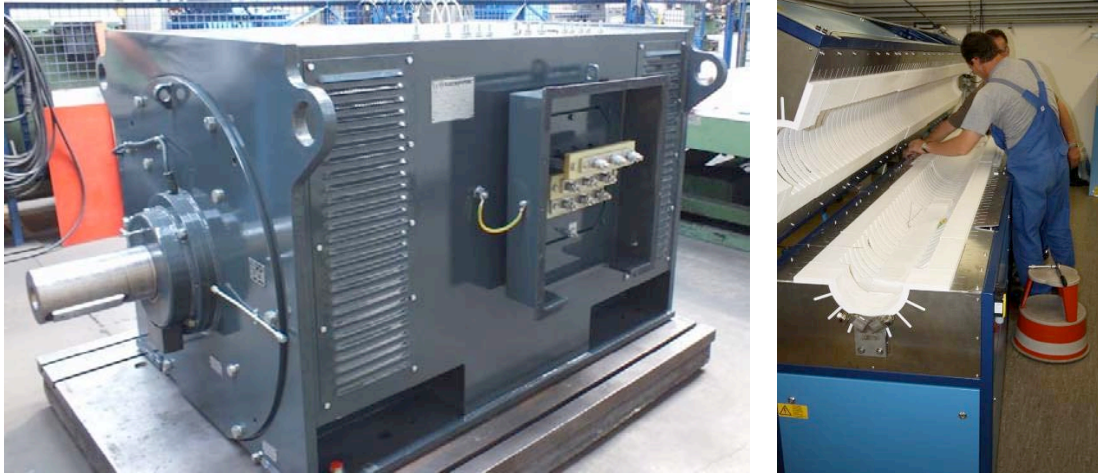
Fig. 3.6.2 The spare motor for the Sultan compressor (left) and the furnace during installation (right).
