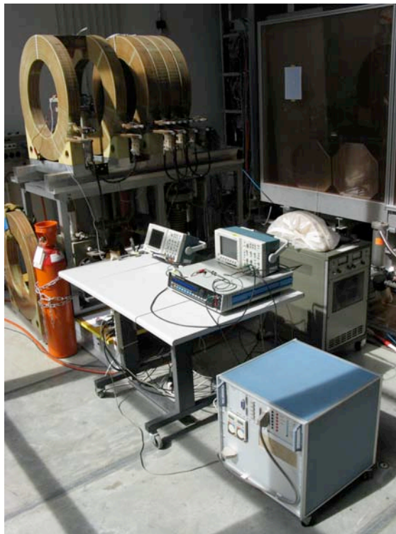
Fig. 4.5.1 Layout of the magnetic axis qualification test inside a Helmholtz coil pair
