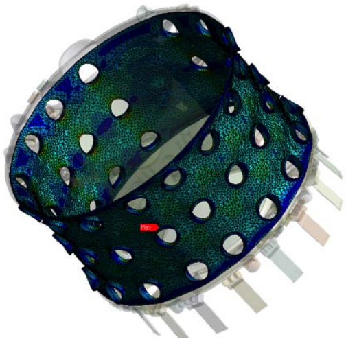
Fig. 3.5.2 Stresses in the outer shell of the TCV vacuum vessel, with plasma disruption loads and atmospheric static pressure applied.
