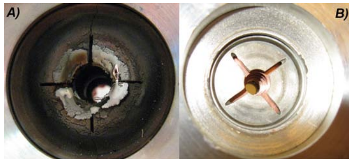
Fig. 3.3.3 “Old” (A) and “re-fabricated” (B) arc-discharge channel with discs (diaphragms)
