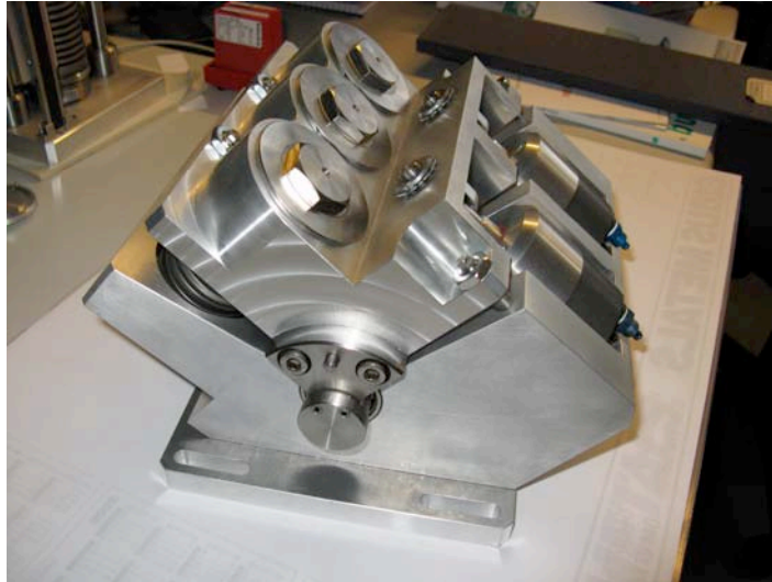
Fig. 4.3.1 The machine springs are held in a special refurbished jig to permit cyclic testing to failure in a heated vacuum chamber mimicking ITER conditions.
