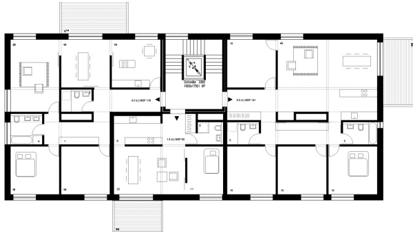
Figure 2: Map of a typical floor resulting from the aggregation of various modules in three apartments with a respective surface of 50 m 2 , 118 m 2 and 141 m 2 .
