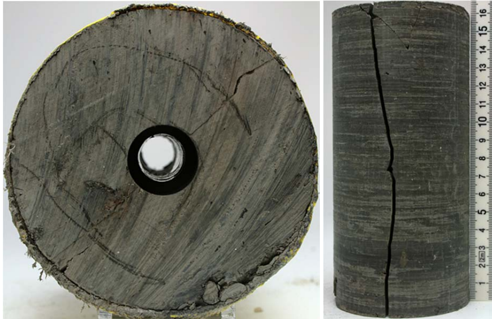
Fig. 9 Pictures before testing of Boom Clay N°14-Bis sample cored perpendicular to bedding in a block retrieved during the Praclay gallery excavation. It was characterised by a distinct fissure close to a diametrical plane
