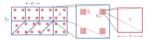
Figure 4.1. Sketch of the FE-HMM algorithm: macro triangulation  $\mathcal{T}_H$  (quadrilateral and simplicial elements) with sampling domains within the macro elements. A close-up of the sampling domains shows the micro triangulation  $\mathcal{T}_h$ , chosen here to be quadrilaterals.
