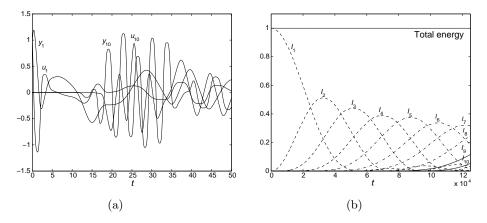
Figure 3.3. The HMM approximation for the solution of the Fermi-Pasta-Ulam equations of motion (3.39) with ten stiff springs, k = 10. (a)  $y_1$ ,  $u_1$ ,  $y_{10}$  and  $u_{10}$  on an O(1) time scale, and (b)  $I_1, \ldots, I_{10}$  on an  $O(\epsilon^{-1})$  scale. The Verlet method takes too long to integrate.
