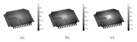
Figure 4.11. Steady-state heat distribution in the three-dimensional microprocessor problem of Example 4, with  $\varepsilon=10^{-6}$  m, 81 000 degrees of freedom in the macro mesh. Comparison of FE-HMM solutions with different resolutions of the micro problems: (a)  $N_{\rm mic}=4$ , (b)  $N_{\rm mic}=8$ , (c)  $N_{\rm mic}=16$ . The bar indicates the temperature in Kelvin (K).
