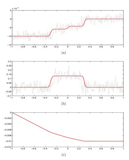
Figure 5.2. Numerical test on shock formation and propagation. 200 macro grid points are used, and each local MD simulation consists of  $40 \times 10$  atoms and  $10^4$  steps of time integration. The solution is displayed after 40 steps of integration over macro time steps. Solid line, computed solution; dashed line, full atom simulation (one realization). (a) Strain, (b) velocity, (c) displacement.
