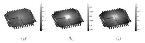
Figure 4.10. Steady-state heat distribution in the three-dimensional microprocessor problem of Example 4, with  $\varepsilon=5\times10^{-4}$  m, 81 000 degrees of freedom in the macro mesh. Comparison of various solutions. (a) Averaged tensor (arithmetic mean), 81 000 degrees of freedom, (b) FE-HMM solution, 81 000 macro degrees of freedom, (c) fine-scale solution,  $3.9\times10^6$  degrees of freedom. The bar indicates the temperature in Kelvin (K).
