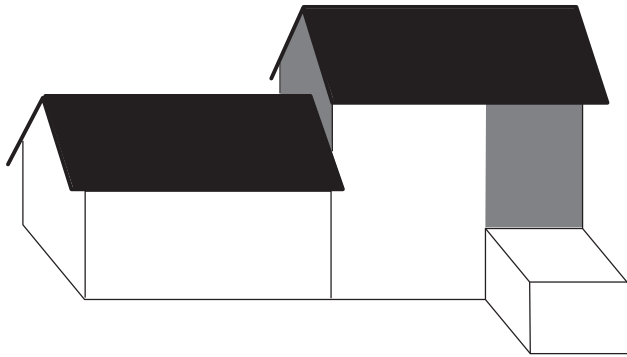
Fig. 1. Typical cases of attached buildings where inner facades (marked in grey) are present.
