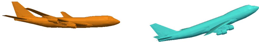
Figure 3.2: Visualization of the different displacement components defining the final configuration: deformative (left-orange) and rigid (right-blue) components.
