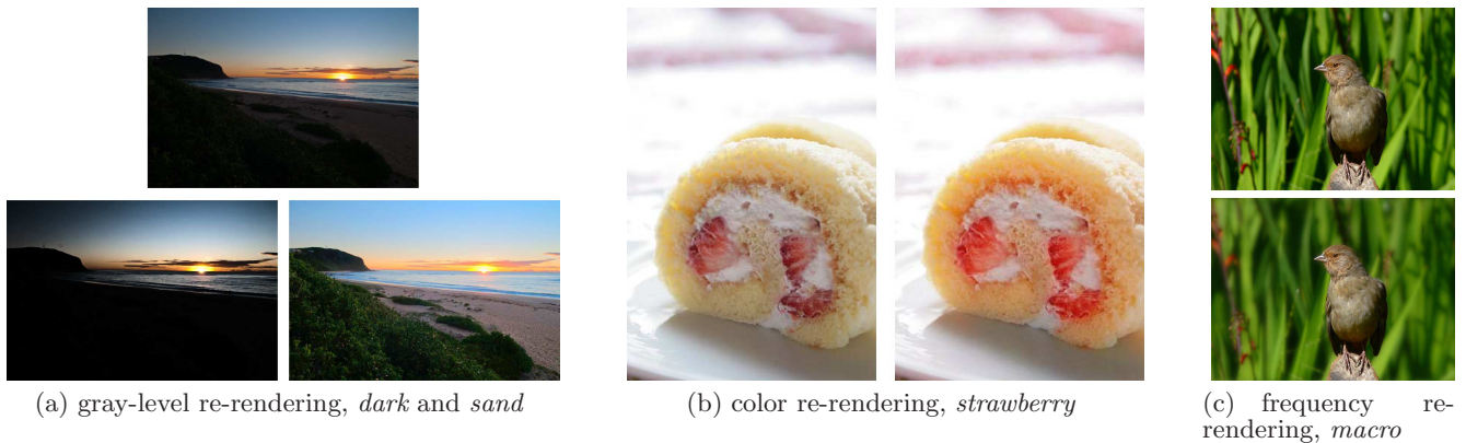
Figure 1: Examples for the three semantic image enhancement algorithms presented in this paper. All algorithms take as inputs a single image and an associated semantic expression, which is indicated in the sub-caption in italic . Left: The gray levels of the input image at the top are tone mapped to adjust for the semantic concepts dark and sand . Middle: The input image’s colors are re-rendered in order to emphasize the concept strawberry . Right: Defocus magnification to adapt to the semantic concept macro . The input image (top) is reproduced from Zhuo and Sim [30].
