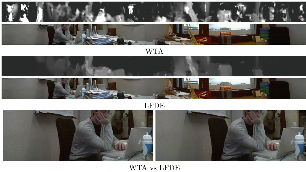
Figure 6.11: Dense depth estimation using the Panoptic Ring camera. The WTA estimation is noisy on untextured area and causes geometric artifacts in the rendered image.
