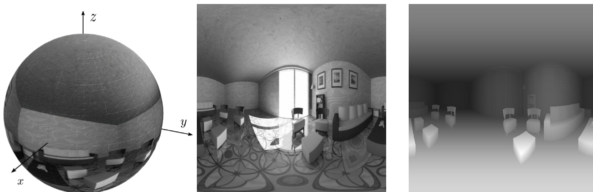
Figure 5.5: The synthetic spherical image. Middle: geographical projection. Right: depth map ground truth
