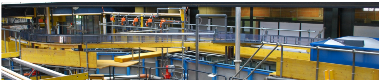
Figure 4: Overview of the physical model with Lake Geneva tank on the right, Veytaux 1 powerhouse in the background and Veytaux 2 powerhouse on the far left
