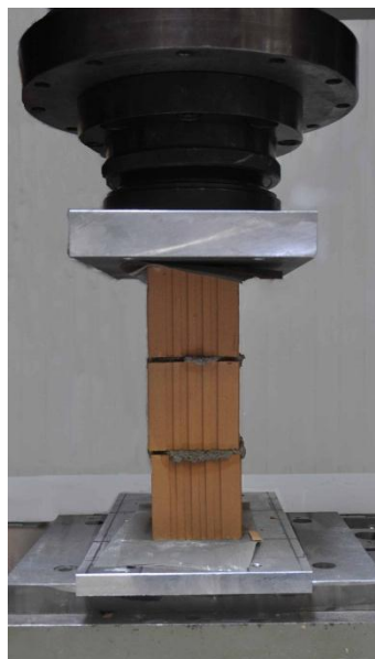
Figure 5.2. Unidirectional compression test on one 1:2-scale masonry triplet.
