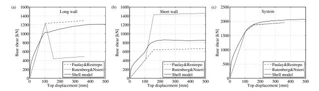
Figure 4.4. Force-deformation relationships of the coupled individual walls and of the system: comparison of numerical results obtained with the shell element model and the two analytical models.
