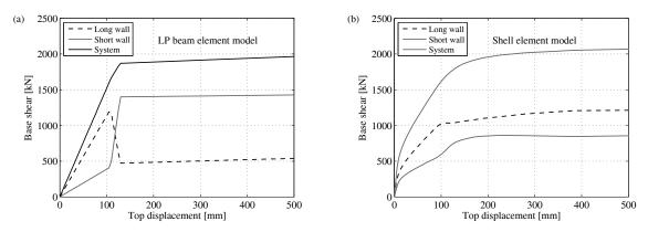
Figure 4.5. Comparison of the force-deformation relationships obtained for the coupled system with the numerical models: (a) lumped plasticity beam element model, (b) shell element model.
