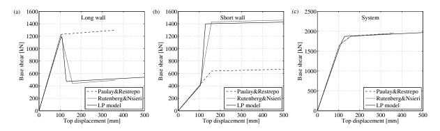
**Figure 4.2**. Force-deformation relationships of the coupled individual walls and of the system: comparison between numerical results obtained with the lumped plasticity beam element model (LP model) and the two analytical models.
