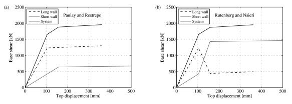
Figure 3.1. Force-deformation relationship of the long and short wall and of the system derived using two analytical models: (a) Paulay and Restrepo, (b) Rutenberg and Nsieri.
