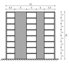
Figure 2.1. Geometry of the planar example structure comprising two walls of different length. All dimensions are in *m*.
