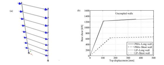
Figure 4.1. (a) Screenshot of the coupled wall system with the lumped plasticity model in Seismostruct.(b) Force-deformation relationships of the single walls obtained: Comparison of the results obtained with the numerical model and the results obtained from the plastic hinge analysis.
