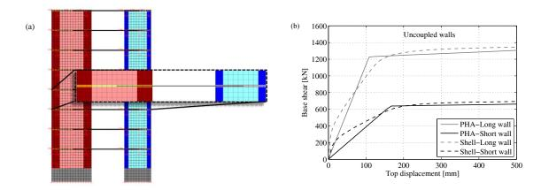
**Figure 4.3**. (a) Screenshot of the coupled wall system model in VecTor2 including detail for the rigid connection model. (b) Force-deformation relationships of the single walls: Comparison of the results obtained with the numerical model and the results obtained from the plastic hinge analysis.
