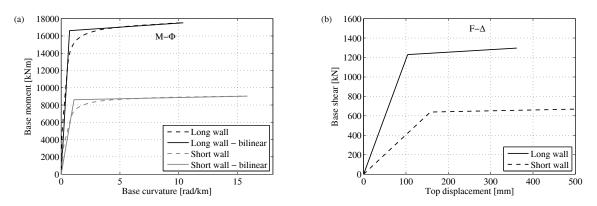
**Figure 2.2**. (a) Moment-curvature relationship of the individual walls including the corresponding bi-linear approximations. (b) Force-deformation relationship of the individual walls.
