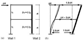
Figure 3.2. Two storey system: (a) Properties and loading, (b) assumed deflected shape and resulting floor forces and base shear forces (Rutenberg, 2004).
