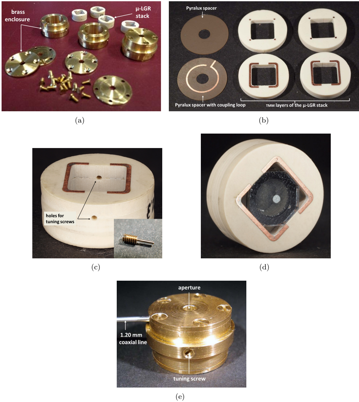
Figure 5.7: (a) Some of the built prototypes, (b) manufactured layers for the cavity stack, (c) the \mu -LGR showing the holes for the tuning screws (inset show one of the 5-mm long tuning screws), (d) assembled \mu -LGR (the outer diameter is 12 mm) containing the miniature Rb cell (e) brass enclosure: the feeding coaxial, one of the cavity apertures and one of the tuning screws are visible.
