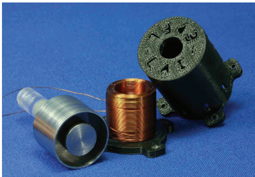
Figure A.4 – Cylindrical actuator parts
