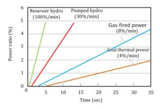
**Figure 7**: Comparison of the adjustable load rates of four power plants [10]
