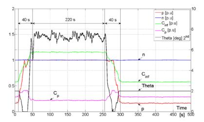
Figure 9: Time history of the wind farm parameters during the wind evolution
