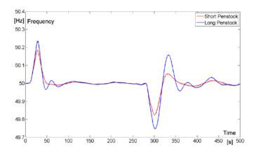
Figure 12: Time history of the network frequency for a long and a short penstock
