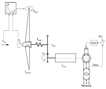
**Figure 3**: Wind turbine model
