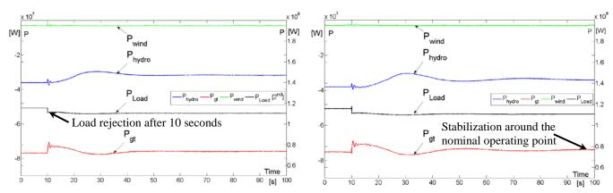
**Figure 16**: Transient behavior after a load rejection for a short penstock
