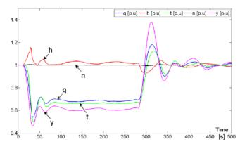
**Figure 13**: Transient behavior of the hydraulic turbine parameters during the wind evolution for a short penstock
