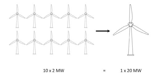
Figure 4: Wind turbine farm of 10 x 2 MW modeled as an equivalent wind turbine of 20 MW
