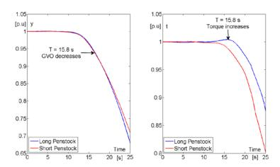
**Figure 15**: Time history of the guide vane opening y and the torque T for the hydraulic turbine
