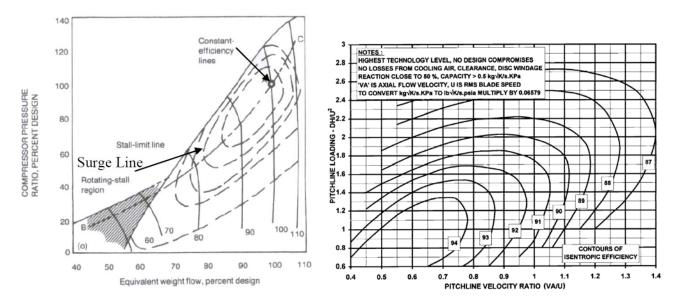
Figure 6: Performance maps of a compressor (left) [8] and a turbine (right) [9]
