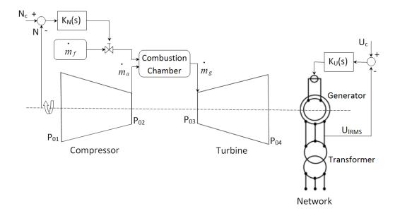
Figure 5: Gas-fired turbine model
