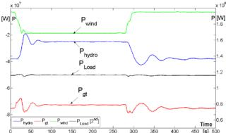
Figure 11: Transient behavior of the active power during the wind evolution for a long penstock
