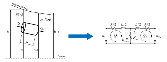
Figure 1: Representation of an elementary hydraulic pipe of length dx and its equivalent circuit
