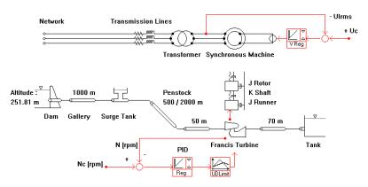
Figure 2: Hydraulic power plant model
