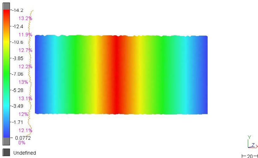
Figure 5.25: Displacement inspected by surface-based approach (3DReshaper)
