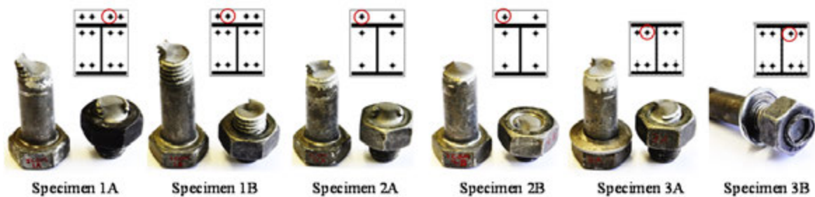
Figure 8. Beam-column connection bolt failures.
