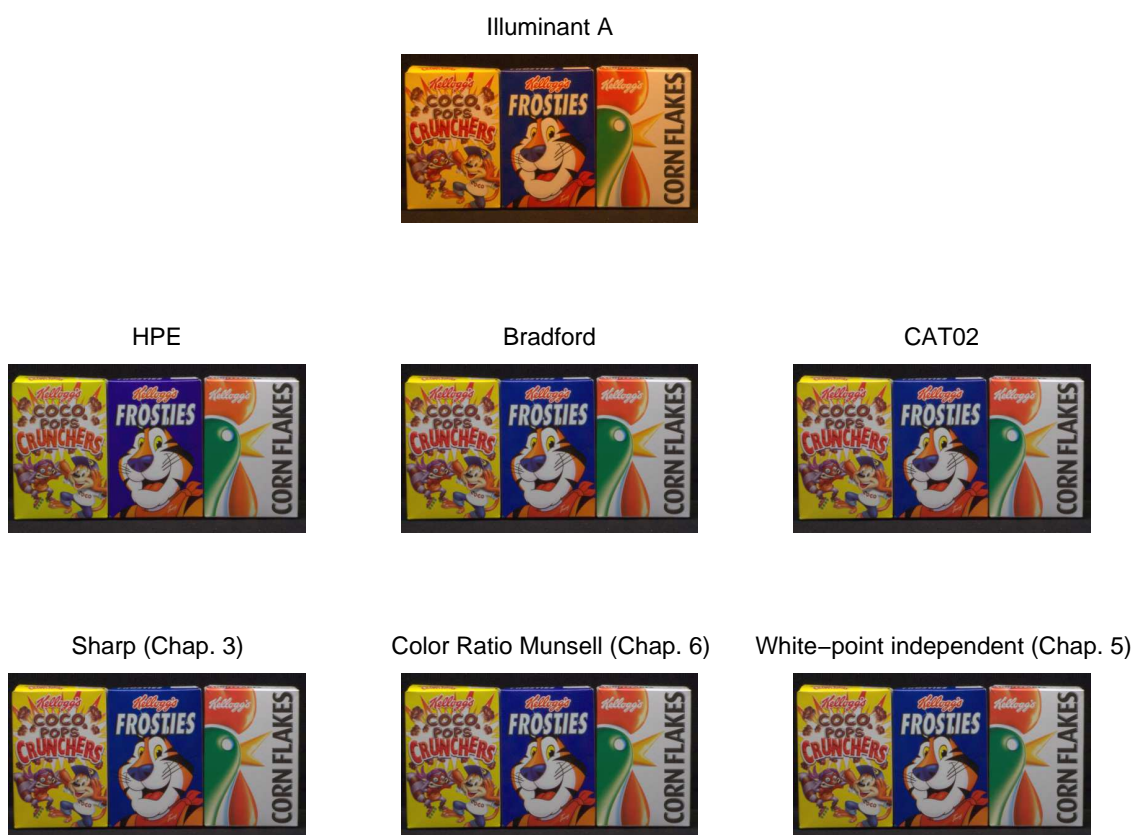
Figure G.3: An image “captured” under illuminant A and rendered to D65 using the different transforms discussed in this thesis.
