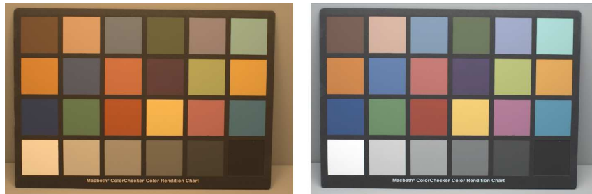
Figure 1.2: Left: An object imaged under a tungsten illuminant. Right: The same image transformed to appear correctly under monitor viewing conditions.
