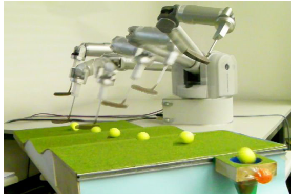
Figure 12: The hitting motion on the WAM. The ball and the hole are continuously tracked by a stereovision system (hence the attached red ball to the hole).
