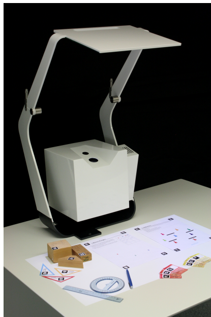
Fig.1: Our camera-projector on a table, along with various types of objects which can be augmented: sheets, cards, tools and wooden blocks.
