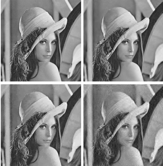
Figure 2. Reconstruction example for Lena in spread spectrum acquisition setting ( M = 0.2N , \text{ISNR} = 30 dB). From left to right and top to bottom: original image, reconstructed images for SARA (28.1 dB), RW-TV (26.3 dB) and BPDb8 (21.4 dB).
