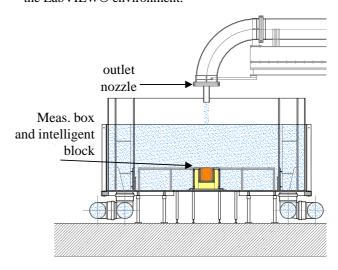
Figure 2: Side view of the experimental facility (Federspiel et al. 2009)
