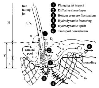
Figure 1: Main parameters and physical-mechanical processes (Bollaert, 2002)
