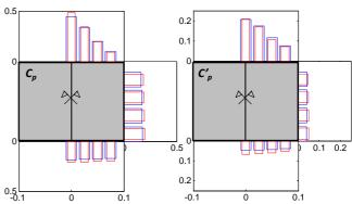
Figure 5: Scaled plots of Cp and  $C_p$ ' around block.  $Y/D_i=11.11$ ;  $V_i=19.65$  m/s. Red: without air. Blue: with air.
