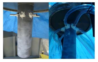
Figure 3: Photos of the nozzle with aluminium tubes installed for air entrainment. In the left, flexible tubes for measurement of entrained air
