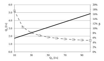
Figure 4: Passively entrained air discharge (black line) and air-water ratio (dashed grey line) as a function of the water jet discharge
