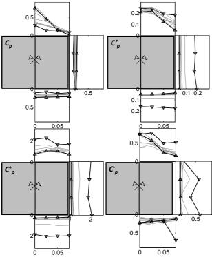
Figure 6: Scaled plots of Cp,  $C_p$ ,  $C_p$ ,  $C_p$  and  $C_p$  for all  $V_j$  around block. Downward triangle:  $V_j = 2.46$  m/s. Upward triangle:  $V_j = 21.14$  m/s. Intermediate values in grey. Aerated test,  $Y/D_j = 6.94$ .
