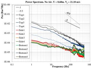
Figure 7: PSD plots for developed jets, with entrained air (top) and without entrained air (bottom).
