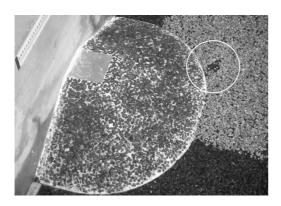
Figure 5 Abutment after a shear failure test.
