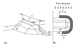
Figure 1 (a) Perspective and (b) schematic plan-view of spill-through abutments
