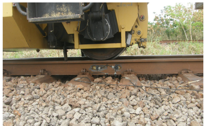
Figure 4. Instrumentation for measurement of axle loads on track.
