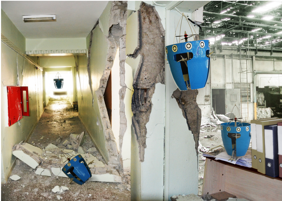
Figure 1.1: An artist's impression of the inside of a damaged building. The ability of flying robots to access elevated areas and pass over rubble on the ground make them uniquely suited for exploring such environments.
