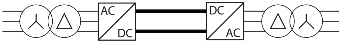
Figure 5.1: Point-to-point connection of a HVDC line based on MMC
