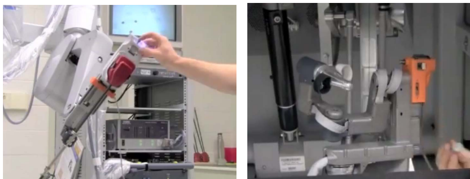
Figure 2.15: The Verrotouch system is composed of two parts: (left) the impact sensors assembled on the slave and (right) the vibrators assembled on the da Vinci surgeon's console McMahan et al. (2011a)
