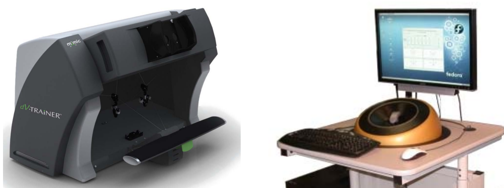
Figure 2.11: (left) dV-Trainer TM , simulator of the da Vinci Surgical system with force feedback capabilities ( Mimic Technologies, 2011 ) and (right) the magnetically levitated haptic device Maglev 200 TM ( Butterfly Haptics, LLC, 2010 )
