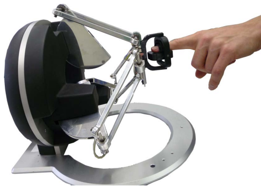
Figure 5.10: Omega.3 device customized with a thimble integrating the tactile pulse display.
