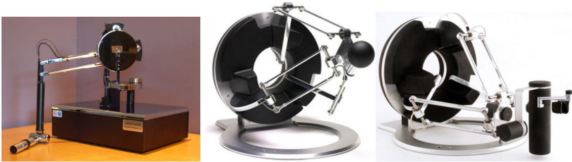
Figure 2.10: Phantom Premium 1.5/6 DOF from Sensable Technologies (2011) , omega.3 and omega.7 haptic devices from Force Dimension (2011)
