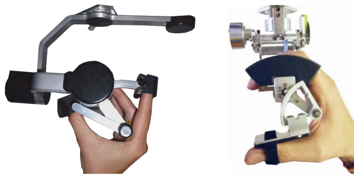
Figure 8.17: (left) standard handle of the omega.7 and (right) the ergonomic handle presented in the previous section.
