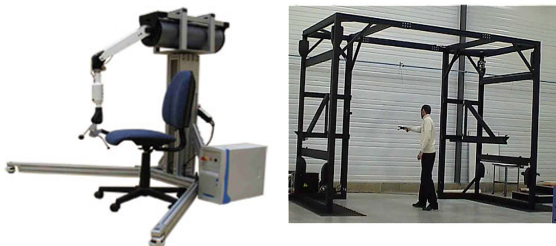
Figure 2.12: High workspace haptic devices for industrial applications from the company Haption SA (2011) : Virtuouse 6D40-40 on the left and Inca TM 6D on the right
