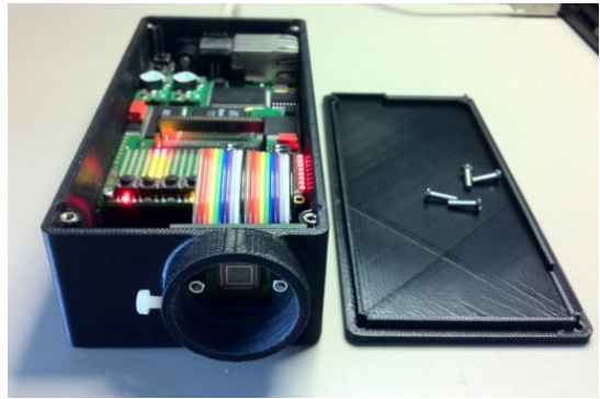
Figure 2: Overall Picture of the custom-designed Camera with Inner Blocks
