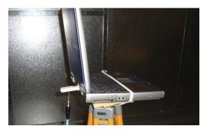
Fig. 2. Reverberation chamber setup for measuring the radiation efficiency of the antenna connected to a laptop computer.
