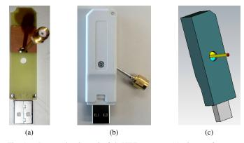
Fig. 1. Improved, microstrip fed, UWB antenna: (a) picture of antenna, (b) USB case, and (c) CST Microwave Studio<sup>TM</sup> model.
