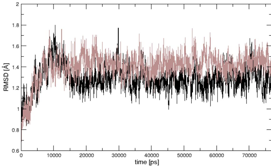
Figure S1: Root-mean-square deviation (RMSD) of backbone atoms from their positions in the initial structure calculated from MD simulations of *apo-Tb6PGL* (black) and *holo-Tb6PGL* (red).
