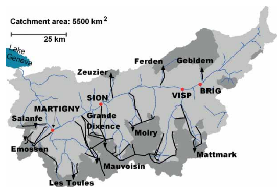
Figure 7 Rhone River basin upstream of Lake Geneva with the 10 major hydropower schemes. The dark grey areas are the drained surfaces by the reservoirs.
