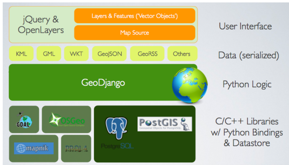
Figure 12: Django specification, Source ref. [21]
