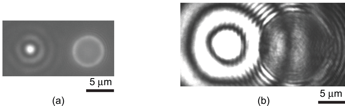
Figure 3. CCD images of the microsphere with the illumination beam aside: (a) 5- \mu m sphere with a Bessel-Gauss beam generated by the NA0.22 objective and (b) 12- \mu m sphere with Bessel-Gauss beam by the NA0.15 objective.
