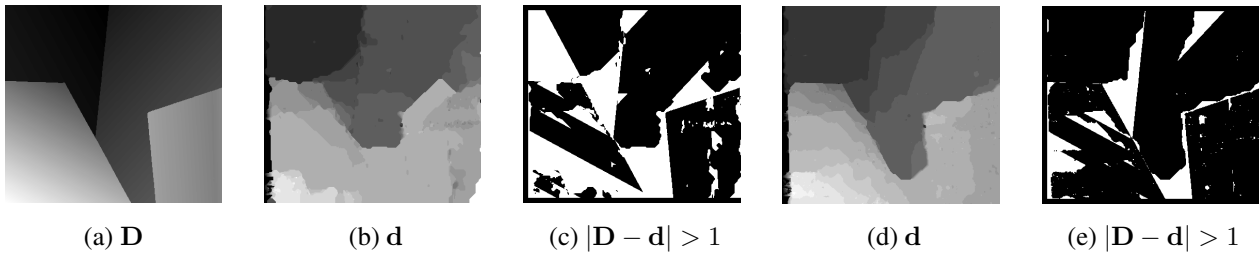
Fig. 3. Comparison of the estimated disparity image from the compressed images with respect to groundtruth information in the Venus dataset. (a) Groundtruth disparity image D ; (b) computed disparity image d at bit rate b = 0.1 ; (c) disparity error at rate b = 0.1 . The pixels with absolute error greater than one is marked in white. The percentage of white pixels is 28%. (d) Computed disparity image d at bit rate b = 0.4 ; (e) disparity error at rate b = 0.4 . The percentage of white pixels is 10.4%.
