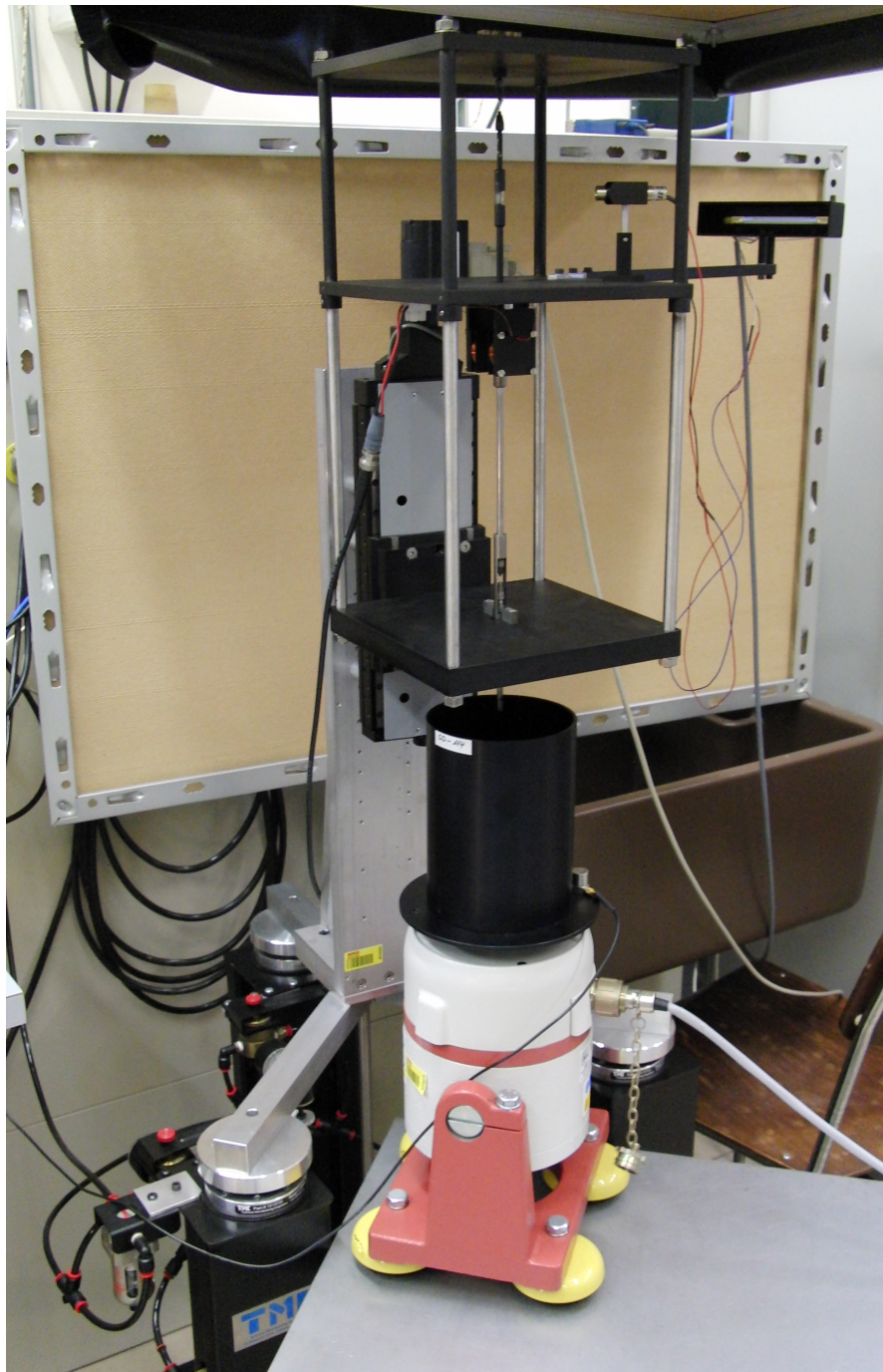
Figure 2.5: Complete view of the torsion oscillator experimental setup. The labels correspond to the ones used in the sketch of Fig. 2.4. This image does not show the electronic chain of measurement that is located in a rack besides the oscillator.
