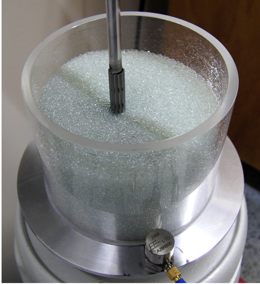
Figure 2.2: Granular sample composed of 1 mm glass beads, in the transparent plastics (PMMA) container. In this case the system is composed of approximately 0.5 kg of glass spheres. The bottom vibrating plate is also visible, with an accelerometer fastened to it.
