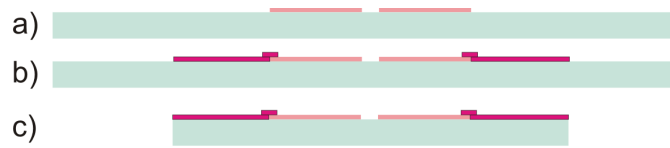
Figure 4.5: Cross-section of fabrication process for electrode chip. ITO electrodes are deposited onto Borofloat substrate (a). Gold is used for the interconnection lines and connection pads (b). The wafer is diced into chips (c).
