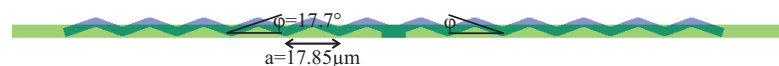
Figure 5.11: A zigzag shaped flap can be fabricated. This zigzag shape can be interpreted as blazed grating with a grating period a and blaze angle \phi . The blue areas indicate the trench and the green areas the torsion beam.
