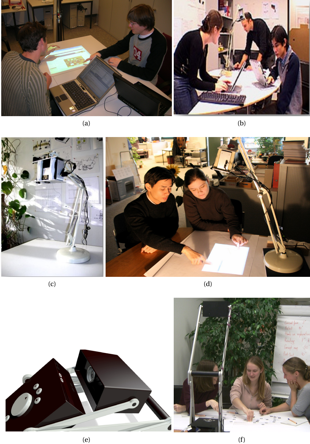
Figure 3.1: (a,b) The first prototype of the DockLamp as a screen sharing device with only a projector in its head, (c,d) The first design of DockLamp as an interactive tangible tabletop system, (e) A Docklamp's industrial design sketch, (f) The final design in use by students.
