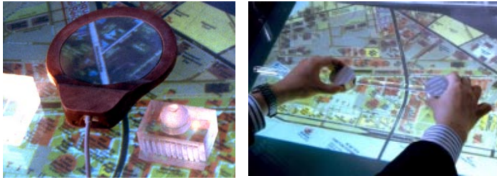
Figure 2.2: The metaDESK (Ishii and Ullmer, 1997) is one of the first tangible user interfaces. Users interact with a set of “phicons” and tangible tools to control a digital map underneath.
