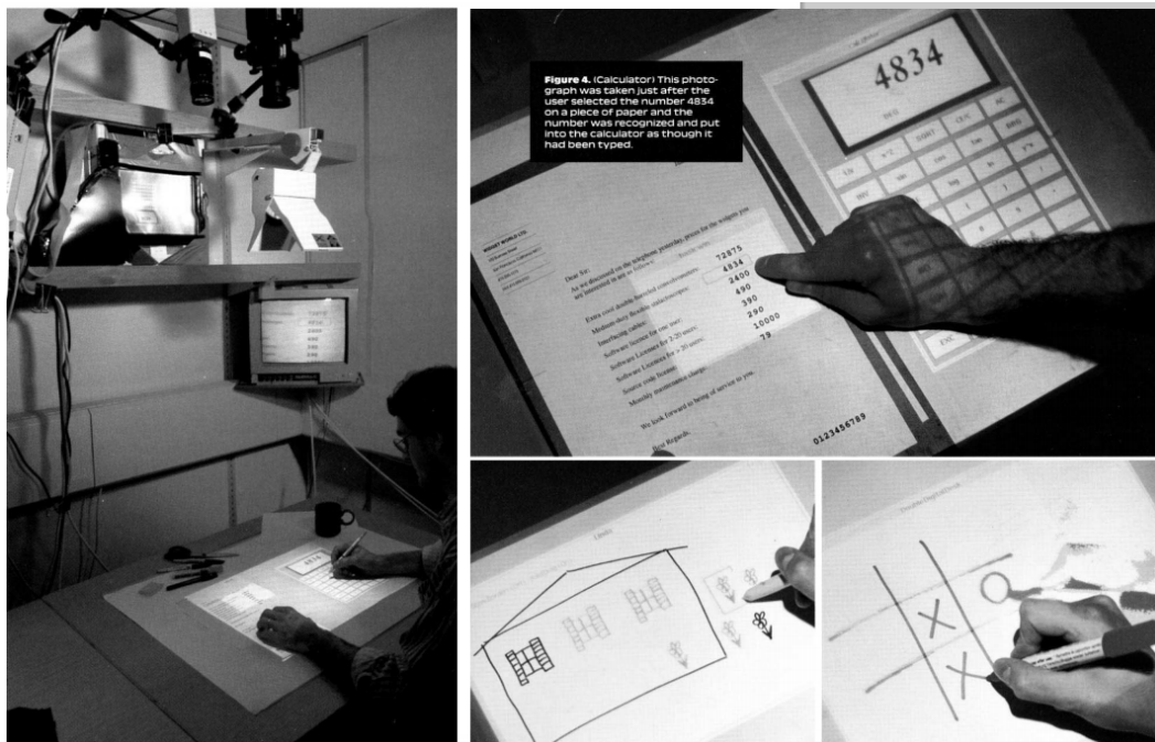
Figure 2.9: The setup of the first tabletop interface: the DigitalDesk (Wellner, 1993).
