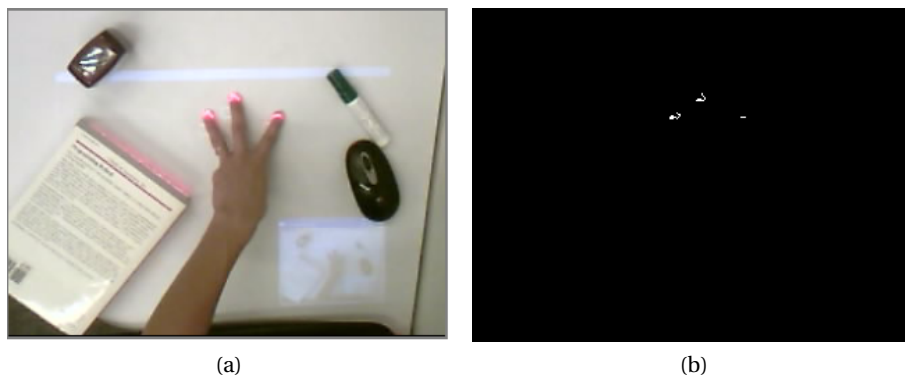
Figure 3.10: Touch detection: a) The red dots appear on fingers when they touch the table b) Detected touches.
