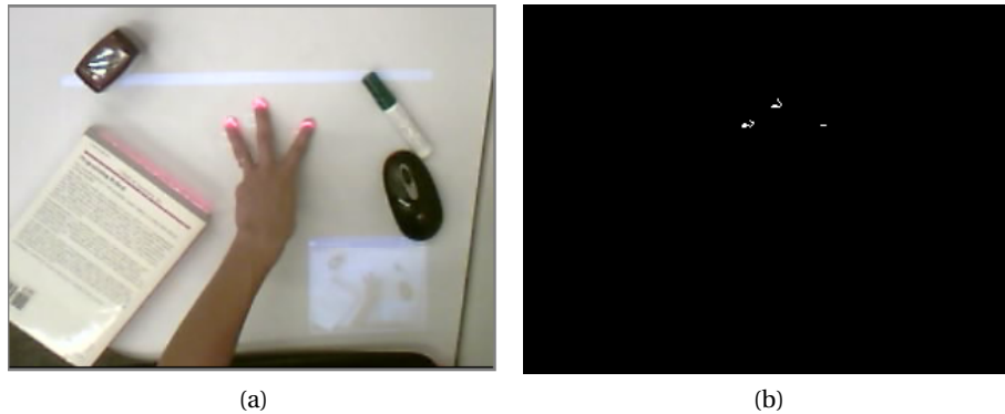
Figure A.4: Touch detection: a) The red dots appear on fingers when they touch the table b) Detected touches.
