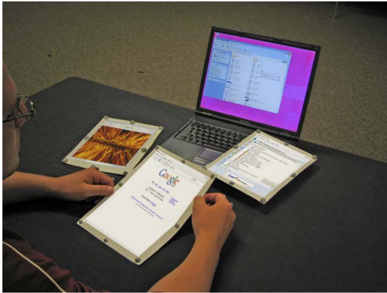
Figure 2.7: The PaperWindow system enables users to use paper to interact with web-browsers (Holman et al., 2005).
