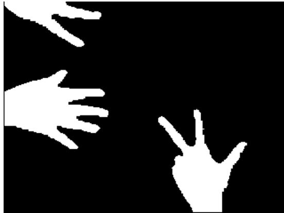
Figure 3.7: A hand mask which was the result of background subtraction, auto-thresholding and skin validation. The white part shows detected hand regions.
