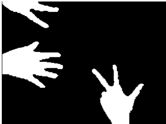
Figure A.1: A hand mask resulted from background subtraction, auto-thresholding and skin validation. The white part shows detected hand regions.
