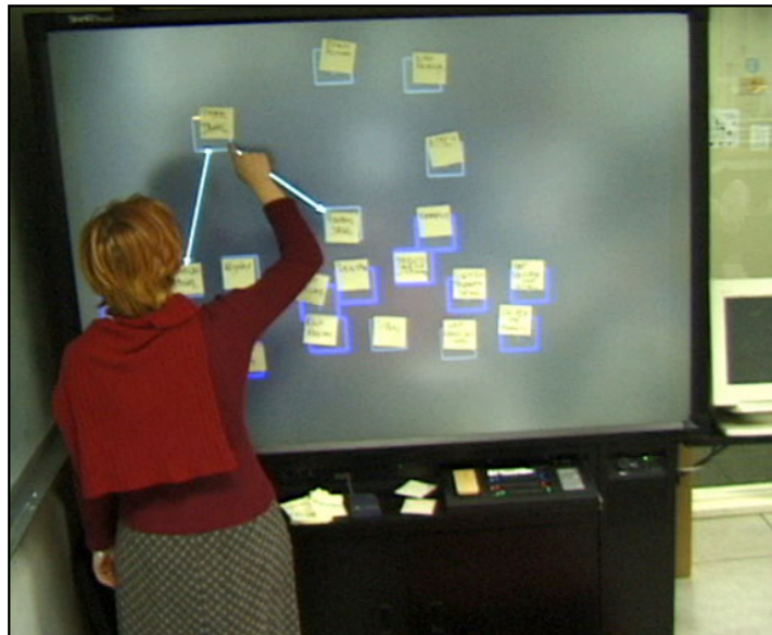
Figure 2.8: Designing websites using post-it paper on the Designers' Outpost system (Klemmer et al., 2001).
