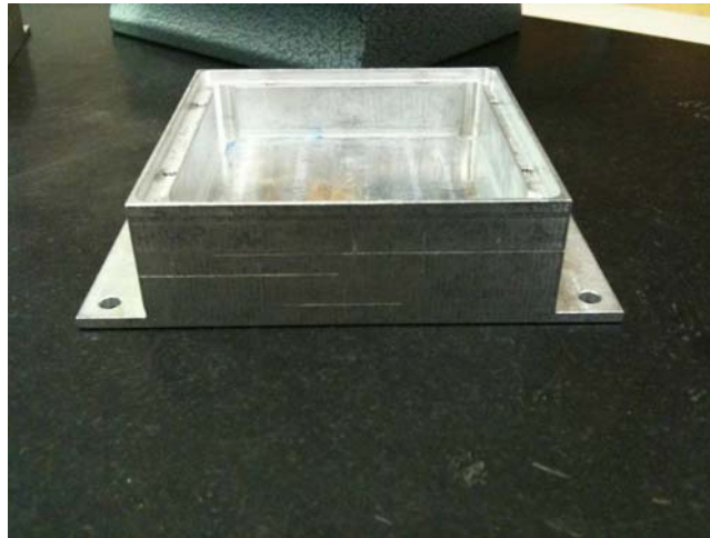
Figure C.50: Shielding box with markings for center of the holes
