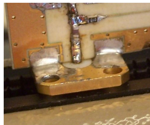
(b) Close view of the SMA once soldered on the PCB
