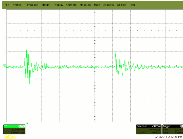
Figure 14.20: The output signal in the time domain for Prototype n° 3 with V_{tune} = (1000000) .
