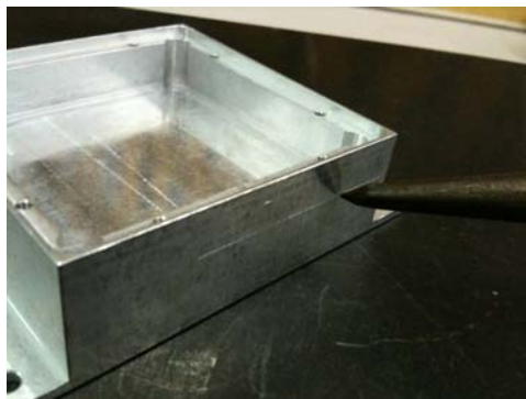
Figure C.49: Marking a line on the shielding box with the marking gauge
