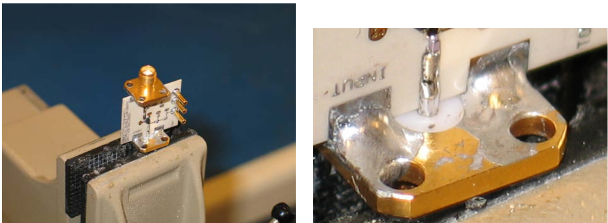
Figure D.7: Large and close view on the single LNA showing how to solder the SMA connectors
