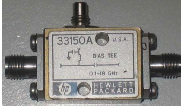
Figure 14.7: The RFC module used powering output stages of Prototype n° 1. The drawing on it is self-explanatory.
