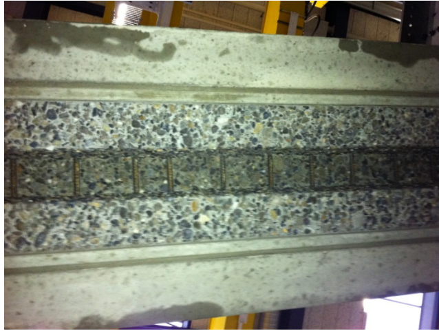
Fig. 3.77: Roughened inner rib of concrete part
