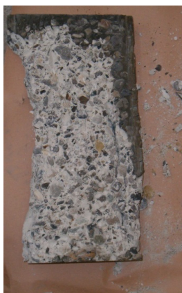
Fig. 3.28: Shear failure inside the concrete block of specimen BR-C_4
