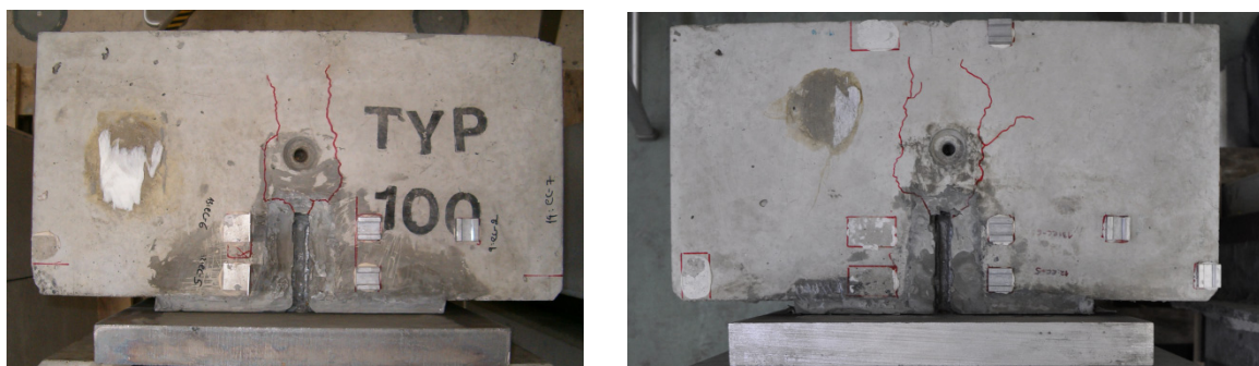
Fig. 3.54: Cracking of concrete blocks at the upper part after failure (specimens PR100_1 & PR100_6).
