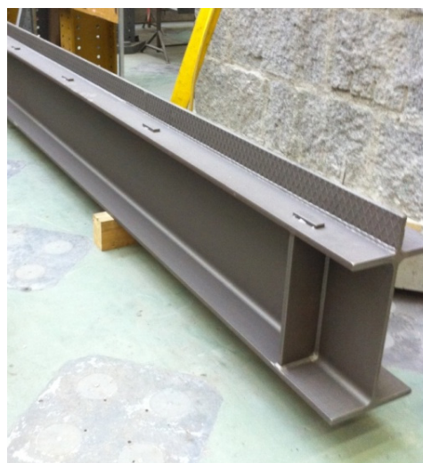
Fig. 3.74: Steel profile HEA 500 and connector of embossed steel plates
