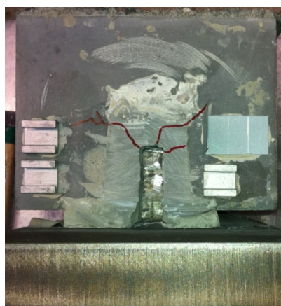
Fig. 3.61 Cracking of UHPFRC block after failure
