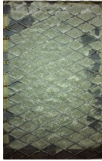
Fig. 3.29: Shear failure in embossed steel-cement grout interface for confinement stress 1 \text{ N/mm}^2 . Cement grout VSL-HPI.
