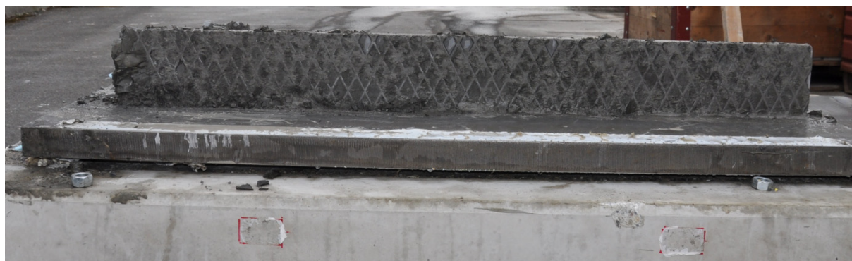
Fig. 3.55: Steel connector after diamond cutting of block, specimen PR100_5.
