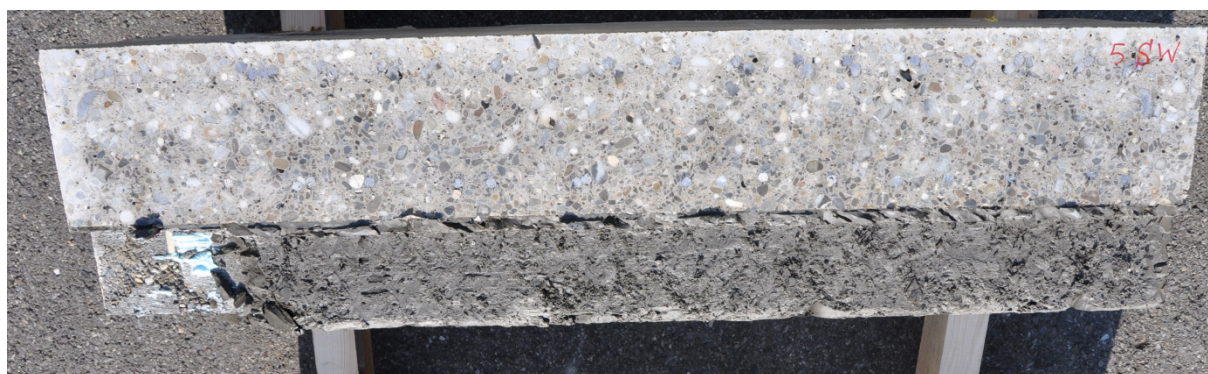
Fig. 3.56: Concrete block after diamond cutting. Cement grout remains attached to rough concrete. Specimen PR100_5
