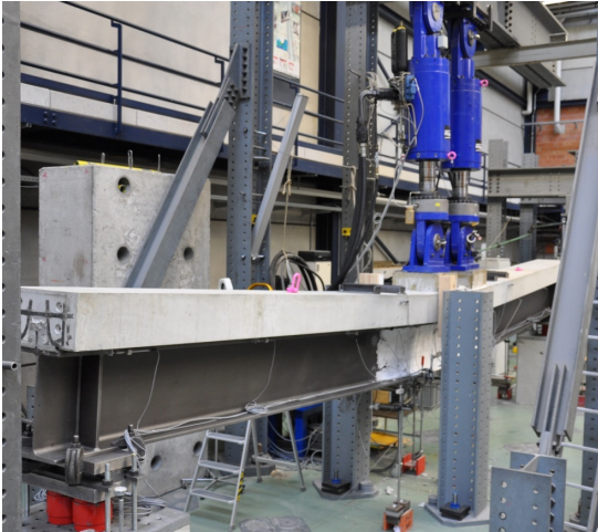
Fig. 3.91: Deformation capacity at the end of test before unloading.
