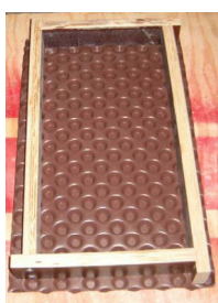
Fig. 3.6 : Form used to produce artificial rough surfaces on UHPFRC with conical studs
