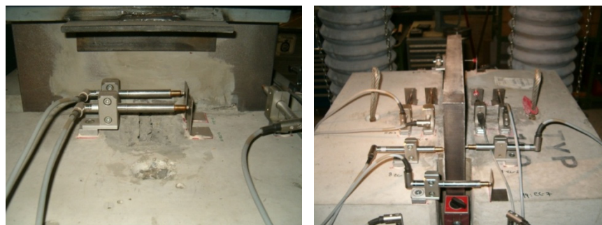
a) Transducers at upper part of reinforced concrete blocks
