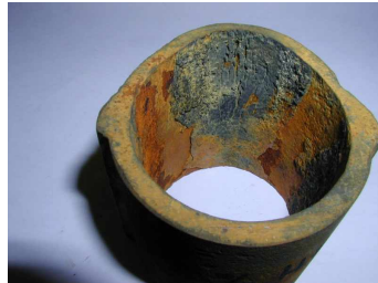
(b) Tube corrosion (source: Power Corrosion Consultants)
