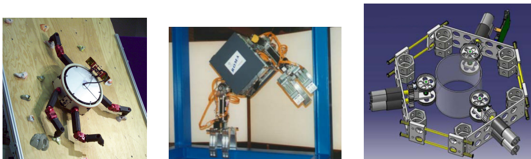
(a) The free climbing Lemur IIb robot (source: [KOA + 06]). (b) The ROMA II robot using claws (source: [BGJ05]). (c) The pole climbing robot from Rodriguez and al. (source: [LBP08]).
