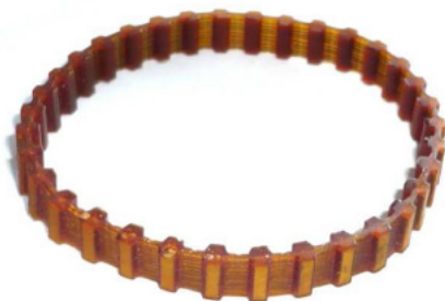
Figure 2.15: Caterpillar embedding magnets. It has a length of 170 mm, a width of 6 mm and thickness of 3 mm.
