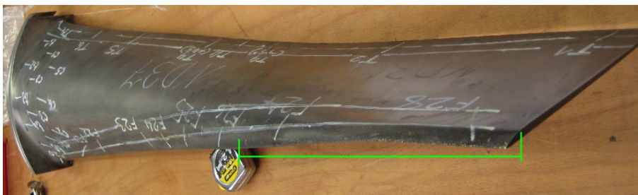
Figure 4.4: ND41A turbine blade. It is 1050 mm long, has a width of 300 mm at the base and 200 mm at the end. It has surface curvatures with radius as small as of 50 mm near the edges. The typical eroded area on the leading edge is shown in green.
