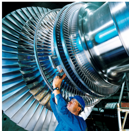
Figure 1.5: Example of steam turbine (source: Wikipedia).
