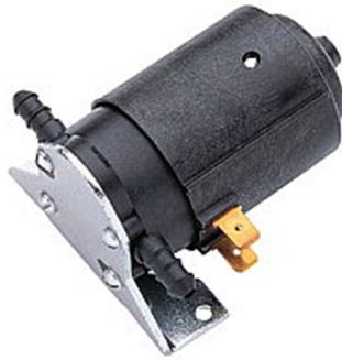
Figure 4.20: Kavan electric pump used to disperse the liquid containing the magnetic particles. It has a maximum flow of 1.8 l/min, and a size of 73x46x60 mm.
