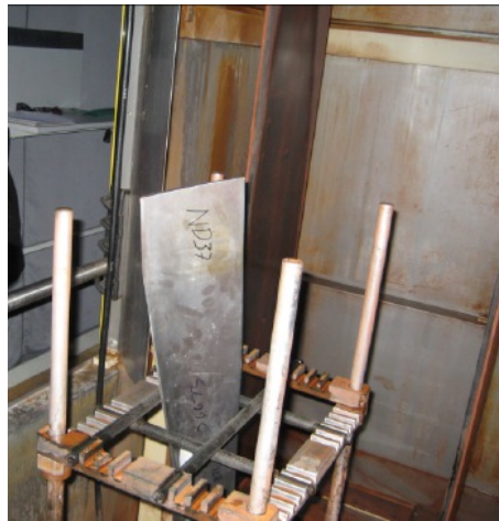
Figure 4.7: Automatic MPI machine at Alstom. Only the final visual inspection is done by the operator.
