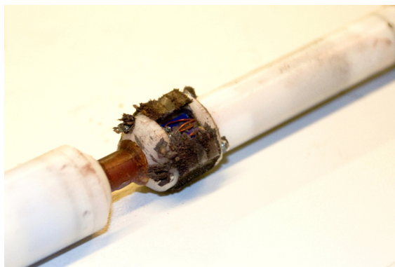
Figure 2.74: Magnetic dust on the MSD. It is easily removable when the adhesion force is switched off.
