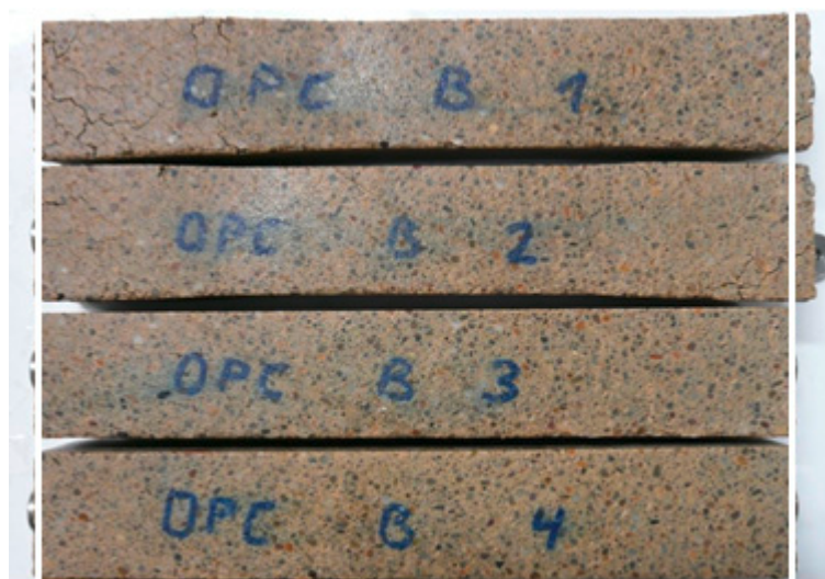
Figure 16: Visual signs of deterioration of the expanding mortar bars were cracking on the specimens ends after 637 days of exposure to sodium bicarbonate solution.
