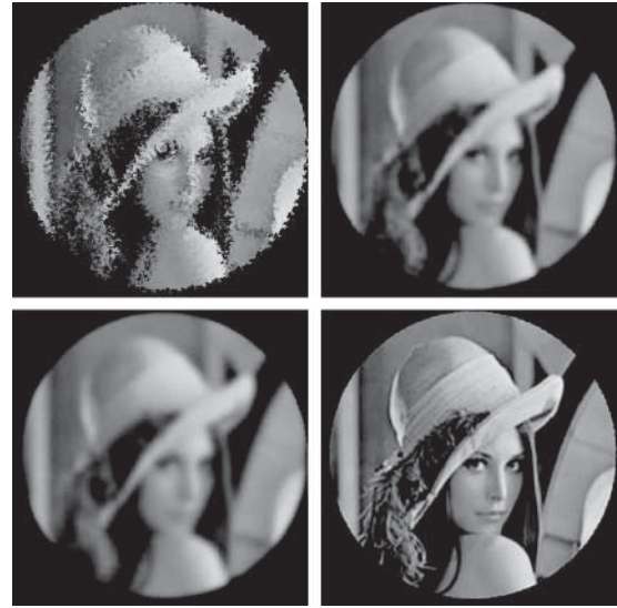
FIGURE 5. The Lena image is rotated repeatedly in 36 steps of 10 degrees each. For every iteration, the outcome of the previous step is interpolated on a rotated grid. Top left: nearest-neighbor interpolation. Top right: linear interpolation. Bottom left: cubic reconstruction without prefilter. Bottom right: prefiltered cubic interpolation.
