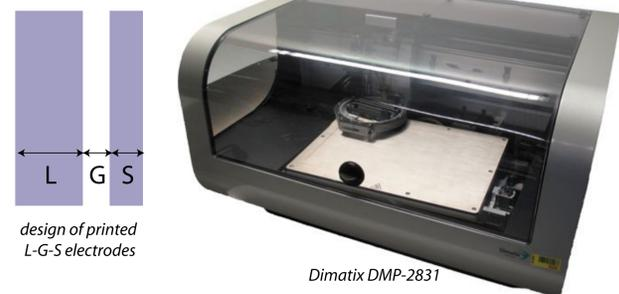
Substrate temperature 40 °C Ink Temperature 30 °C
