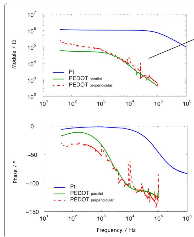
PEDOT:PSS has lower impedance, due to a printed electrode gap smaller than designed
