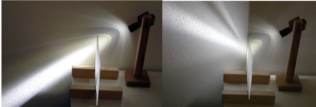
Fig. 6.1 Demonstration of light redirection performance: light distribution without (left) and with inserted daylighting system (right).
