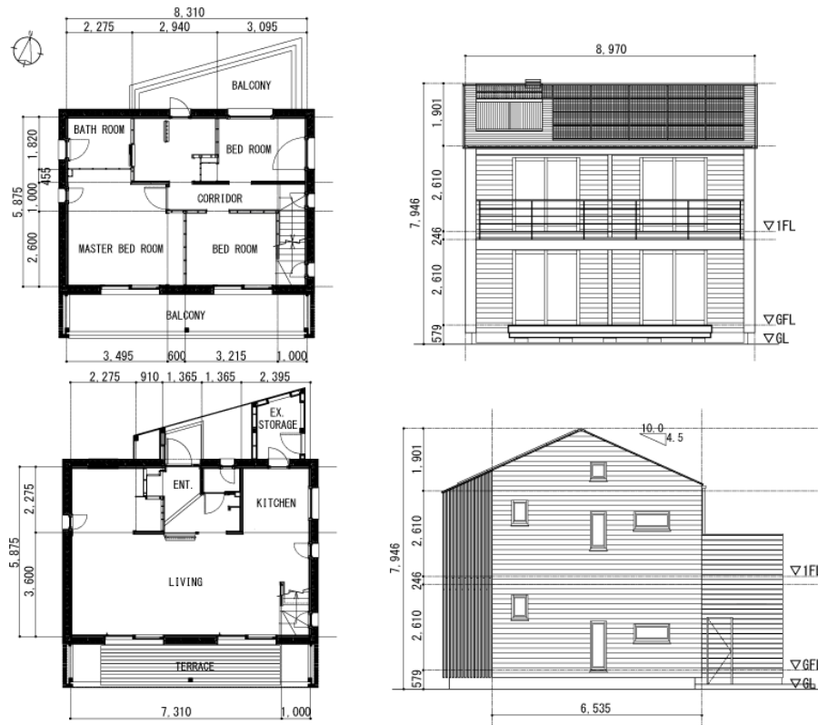
Figure 2: The drawings of Test House (floor plans, elevation plans).
