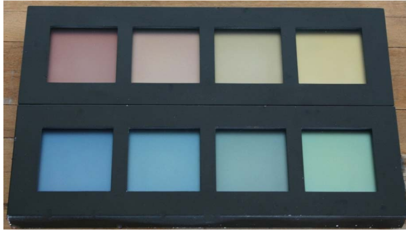
Figure 2: Demonstration boxes with eight homogenous coloured thin-film filters on 4-mm-thick extra white glass samples ( 70 \times 60 \text{ mm}^2 ) with front surface treatment by chemical etching. The coloured filters hide perfectly the parts of a real solar thermal absorber mounted at the bottom of the demo boxes.
