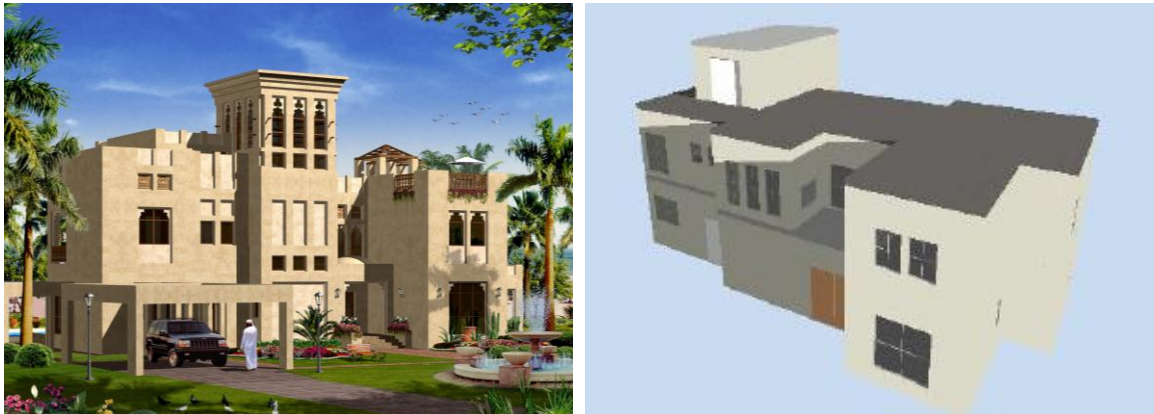
Figure 2: The modelled single family home in Raz al Khaimah. To the right is the 3-D model used for calculations.
