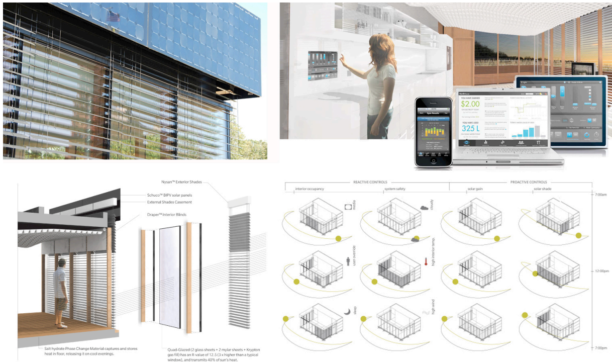
Figure 1: (top left) North House completed façade detail at BIPV cladding and exterior dynamic shading; (top right) User interface components and embedded design; (bottom left) DReSS components diagram; (bottom right) Exterior shade configurations based on climatic and solar data and as prioritized in CHAS logic controls.
