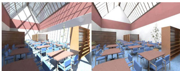
Figure 3: A comparison between clear windows (left) and translucent aerogel windows (right).
