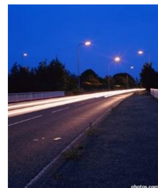
Figure 7: Most night-time outdoor lighting provides illumination in the mesopic region where both rods and cones provide visual information.
