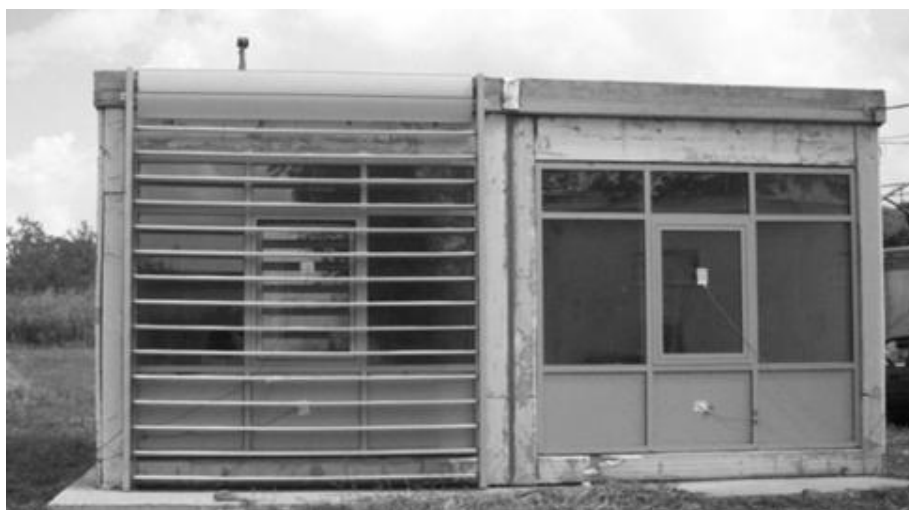
Figure 1: The south side of the experimental cells [3]: Cell A with the integrated blinds on the left and cell B without solar protection on the right.
