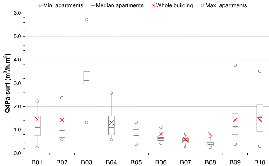
Figure 1: Box plot of the measured air permeability values in each building: the box lines indicate the statistic results of individual measurements and the red marks indicate the global measurement of the whole building in each case. The global measurements of B03* and B05* have been excluded.
