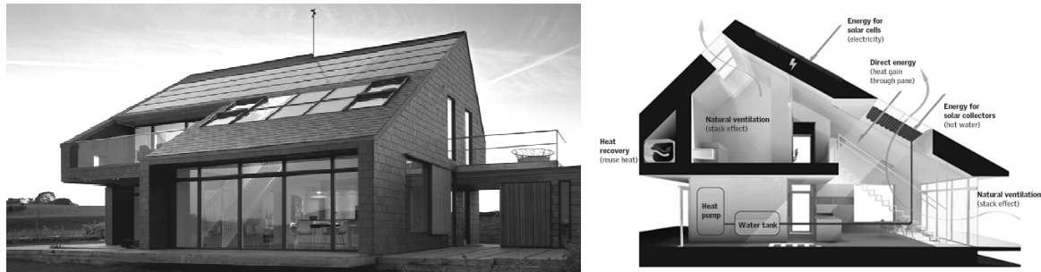
Fig. 1. “Home for Life”. South facade (left). Daylight, ventilation and energy concept (right)
