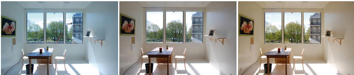
Figure 1: Photograph of the interior of the scaled office room taken from the viewpoint of the research participant. Starting from left to right: views with the blue, neutral and bronze glazing.
