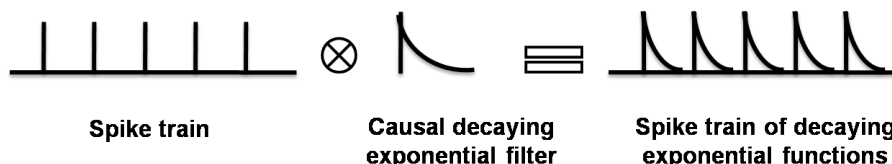
Figure 6.4: The convolution between the spike train of ventricular impulses and the causal one-pole lowpass filter resulting in a continuous signal of decaying exponential functions.
