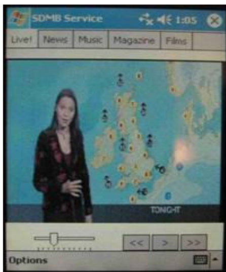
Figure 2: Image of the mobile TV interface. Channel tabs on top, skip forward and back buttons on the lower right with the Pause/Play button in the middle and the audio control slider is located to the left of these buttons.
