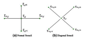
Fig. 6 Updating a grid point: multi-stencil approach
