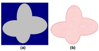
Fig. 11 Arbitrary pocket and contour parallel tool path
