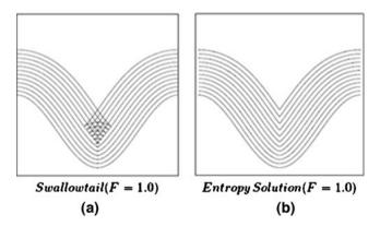
Fig. 4 The evolution of curve a Lagrangian approach b entropybased construction [20]
