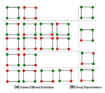
Fig. 8 a Different possibilities for the vertex leveling, *green* points corresponds to point with T value>0 and *red* points show points with value $\leq 0$  b group representation
