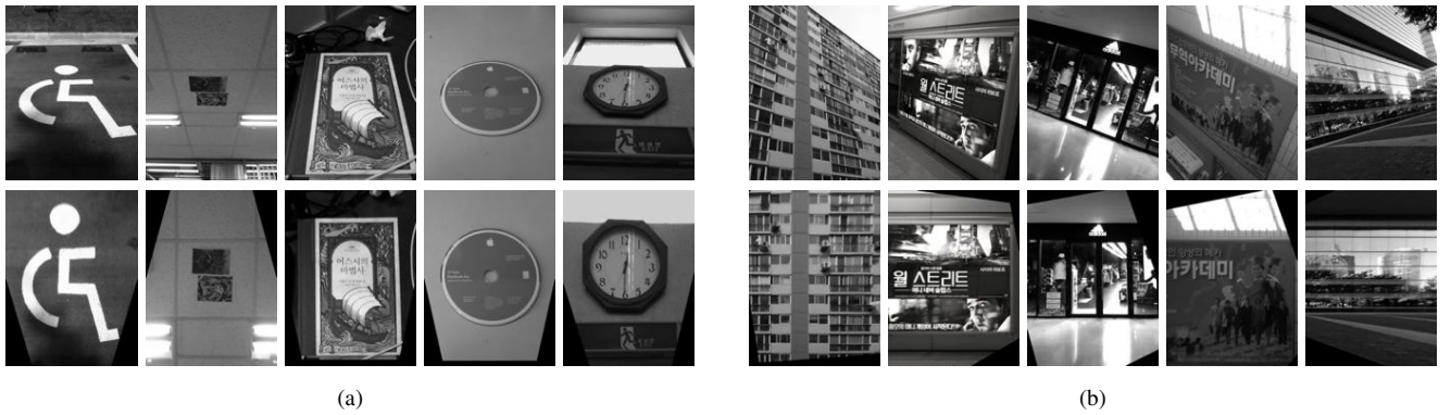
Fig. 8: Examples of estimated fronto-parallel views (bottom row) from different input images (top row). (a) Only the phone accelerometers are needed for horizontal surfaces (columns 1 to 4). It is also true when a vertical surface is rotated in pitch only, as shown in column 4. (b) However, for slanted vertical surfaces, we need to combine the accelerometer’s output with vanishing points detection.
