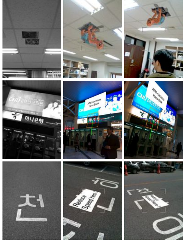
Fig. 1: Overview of our approach. The user simply has to point the mobile phone toward the desired location for the augmentation, and then take a picture like the ones on the left column. Our method guesses the surface orientation for a coherent insertion, by combining the phone’s accelerometers and Computer Vision techniques. It can then recognize the location even from new viewpoints, and track it for real-time augmentation (see middle and right columns).
